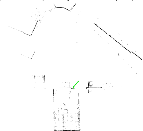
Figure 7: Robot trajectory (green) and map of the environment rendered to the ground plane.
