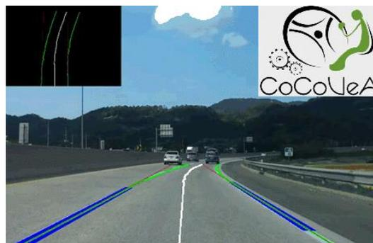
Figure 17: Illustration of CoCoVeA project. Road marking are detected in real time by the autonomous car.
