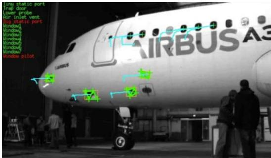
Figure 7: Tracking of visual features for pose estimation.
