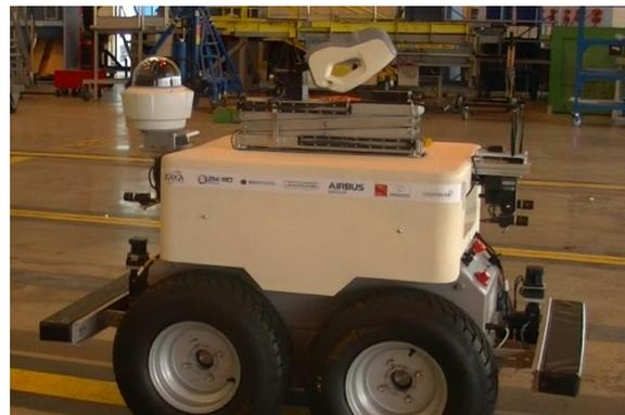
Figure 3: Air-Cobot is equipped with many sensors.
