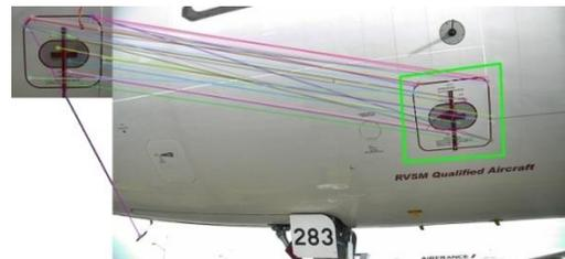
Figure 9: Static port inspection with SURF method.
