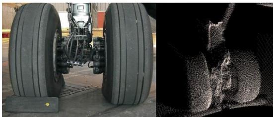
Figure 11: At left, a picture from PTZ camera of a landing gear with a chock in front of the left tire. The task is the detection of the chock. At right, an example of laser data acquisition of a landing gear.
