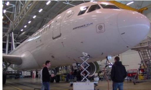
Figure 14: Elevation of the scanner in order to perform a scan of A320 aircraft in a hangar of Air France Industries.
