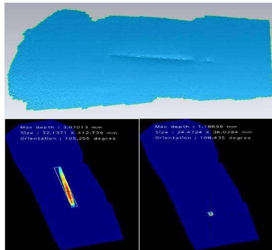
Figure 15: Tridimensional scan of the aircraft, a crack and a bump are visible. The inspection algorithms provide shape, size and depth of those imperfections with visual color representation to help the human operator.
