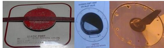
Figure 8: Examples of items to inspect. From left to right, static port with its protection, open air inlet valve, AOA probe. Light conditions are very different.
