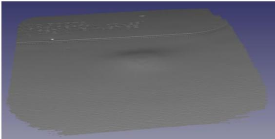
Figure 10: Tridimensional scan of the aircraft surface, a bump is visible in the middle. The writing, visible in the top, helps to locate precisely the default.
