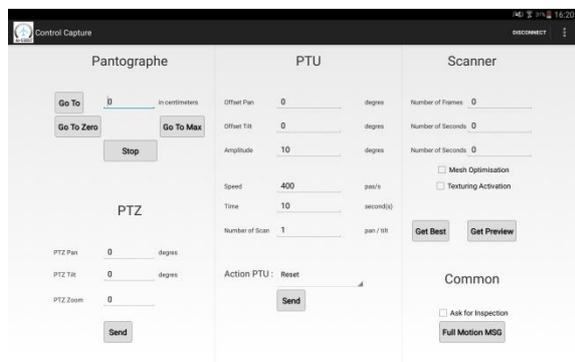
Figure 4: View of the control panel for the NDT sensors.
