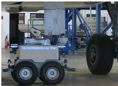
Figure 1: Air-Cobot platform evolving under an A320 aircraft in a hangar of Air France Industries.
