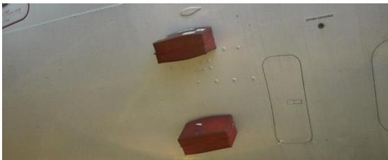
Figure 12: Pitot probe protections are in place.
