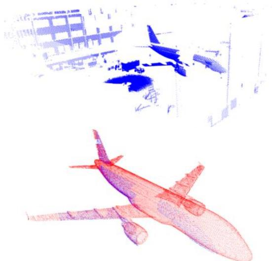
Figure 6: Robot is located in back left of the aircraft in an inside environment. At top, 3D data is acquired with a Hokuyo laser range finder moved thanks to a pan-tilt unit. At bottom, the matching result is made of data (blue) with model (red).
