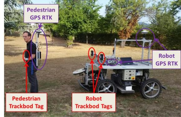
Figure 1: image of the leader and the follower robot both equipped with GPS RTK in order to get the ground truth and to evaluate the precision of the Trackbod system.
