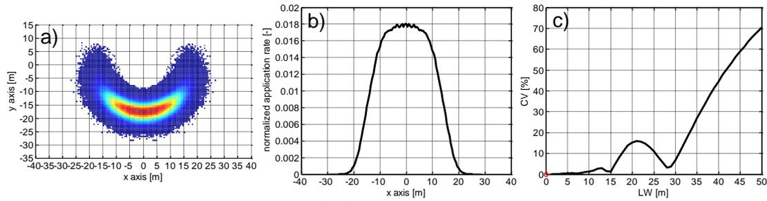
Figure 2 : single spread pattern obtained on a flat field (a) and its transverse application rate curve (b) and CV (c)
