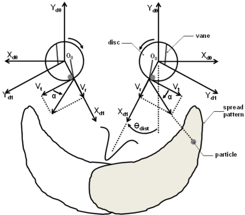
Figure 1: representation of a twin-disc spreader top view and a spread pattern resulting from the overlapping of two single spread patterns.  $\alpha$ , the horizontal outlet angle used in the calculation of the initial output velocities;  $\theta_{dist}$ , the horizontal distribution angle.
