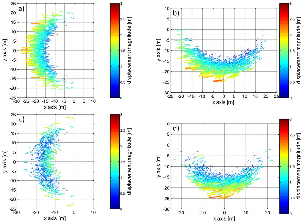
Figure 3 : displacement fields of spread patterns due to 20° slope (a), 20° side-slope (b), 20° slope with 2° Tilt for the discs (c) and 20° side-slope with 2° of side-tilt for the left disc only (d)
