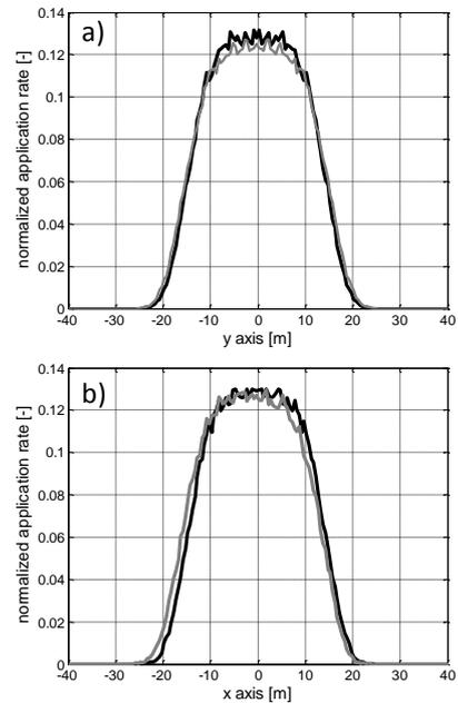
Figure 4 : transverse application rate curves of the spread pattern obtained on a flat field (black) superposed with the one on slope (a) and on side-slope (b) (gray).
