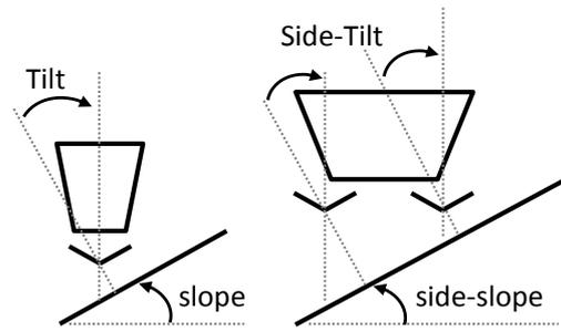
Figure 5 : representation of the tilt and side-tilt corrections applied respectively in the case of slope and side-slope
