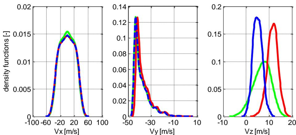
Figure 6 : distributions of particles output velocities on a flat field in the case of 0° tilt and side tilt (blue), in the case of 10° tilt around X axis (red) and 10° side-tilt around Y axis (green)
