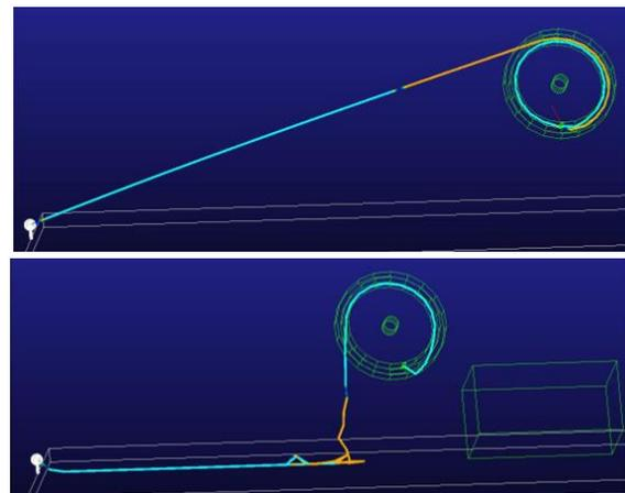
Figure 15:Co-simulation without optimized control: reel speed<vehicle speed (top), reel speed>vehicle speed (bottom)
