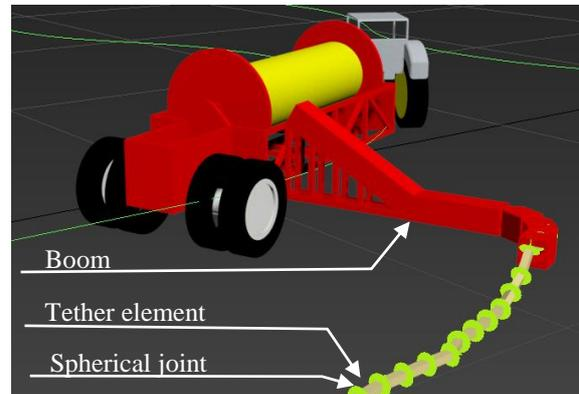
Figure 9: Model of the spreader in physics engines
