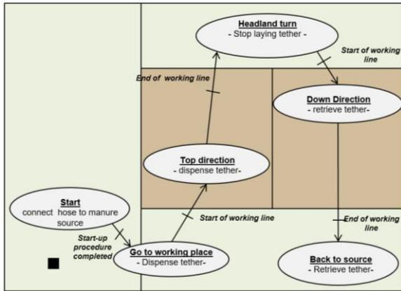
Figure 2 State machine of the tether management system implemented in Simulink
