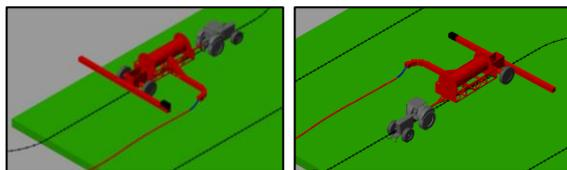
Figure 13 –Slurry spreader dispensing and retrieving the tether: no collision and tension seems no to be too high
