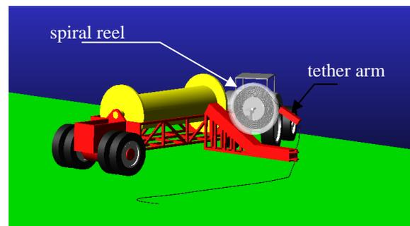
Figure 10 spiral reel and tether arm models connected to the spreader.
