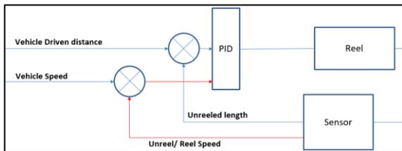
Figure 3 Multivariable PID control implemented in Simulink
