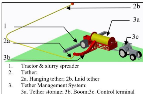
Figure 1: 3D CAD model umbilical slurry spreader from WM Innovations (Ruen, 2010)
