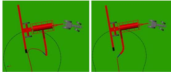
Figure 14 Umbilical Slurry spreader during headland turn maneuver (left: collision; right: no collision)
