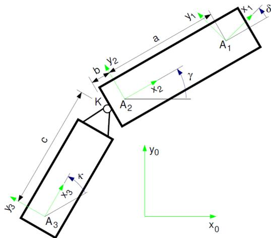
Figure 5: Kinematic model with trailer (Rill, 2006)
