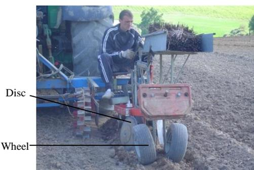
Figure 2: A double disc planting machine hitched up to a tractor.
