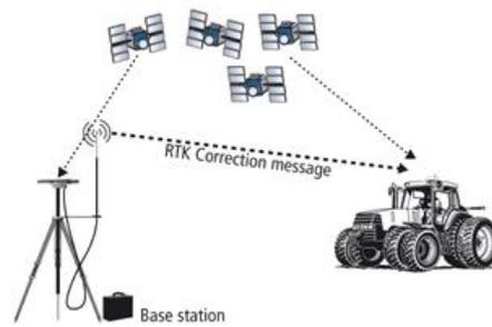
Figure.6. RTK configuration
