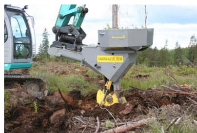
Figure 1: A Bracke planter mounted on an excavator.
