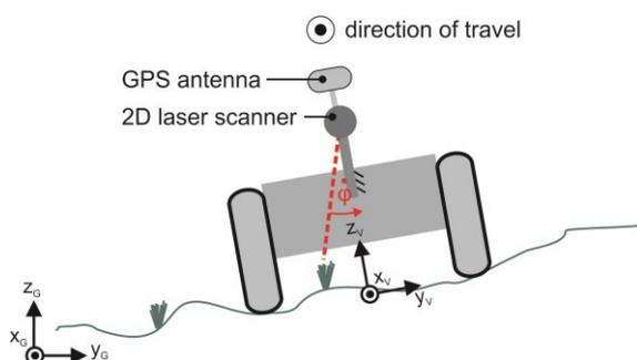
Figure 1: schematic sketch of the pasture robot with attached 2D laser scanner at the front
