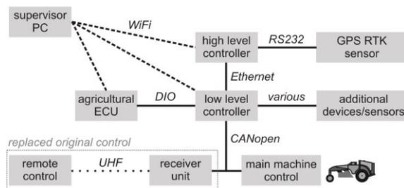
Figure 4: Architecture of the robot
