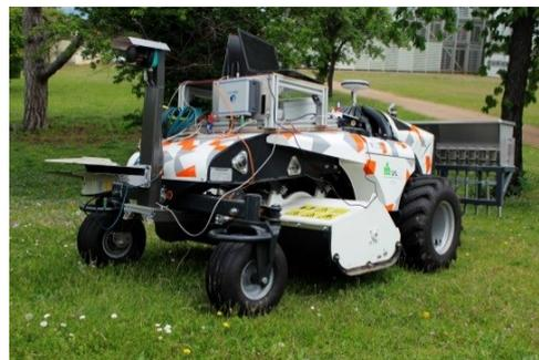
Figure 3: pasture maintenance robot with mulcher and seeder
