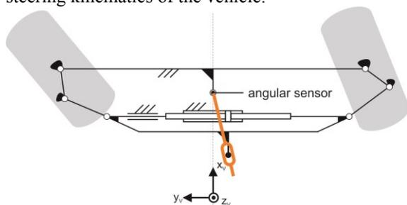
Figure 2: steering kinematics of the robot front wheels
