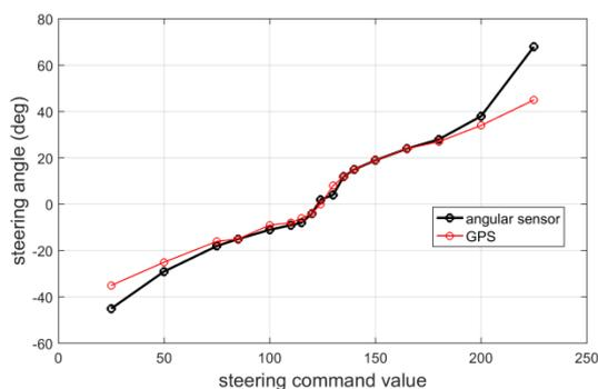
Figure 5: result of steady-state circular tests for different steering command values
