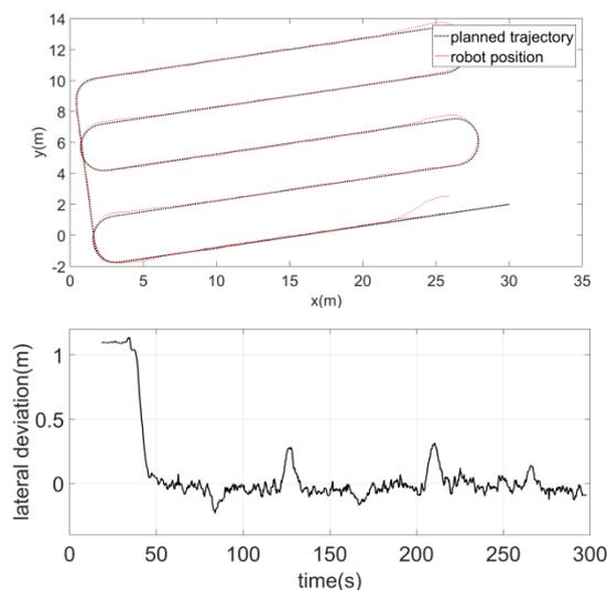
Figure 6: test on grazing area; reference and actual position (top), lateral deviation (bottom)
