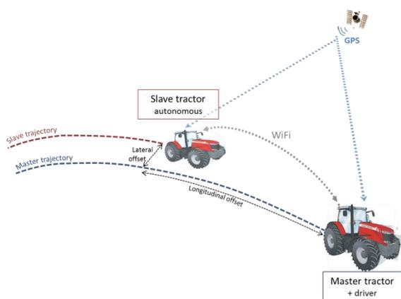
Figure 2. Master-Slave system description.
