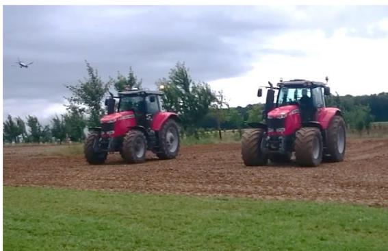
Figure 5. Master (right) and slave (left) tractors in a side-by-side configuration.
