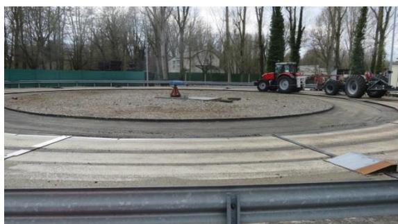
Figure 6. The circular track with bumps.
