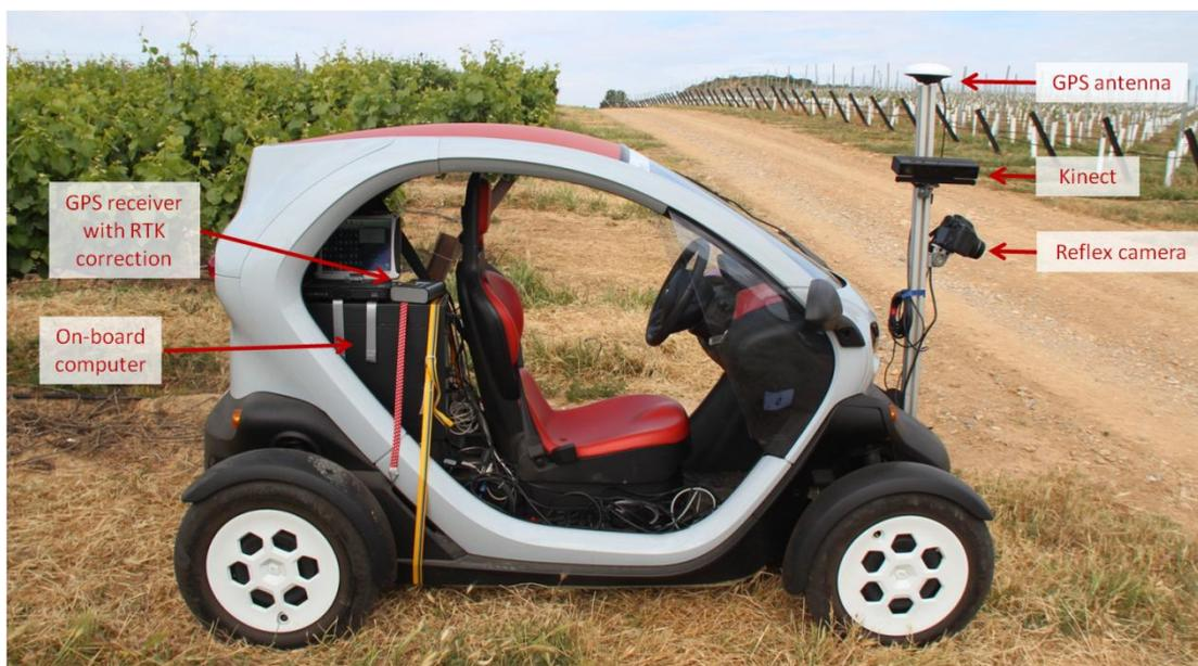
Figure 1 : Electric inspection platform.
