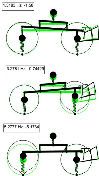
Figure 9: First three calculated eigenmodes of the tractor model with an unsprung rear axle.
