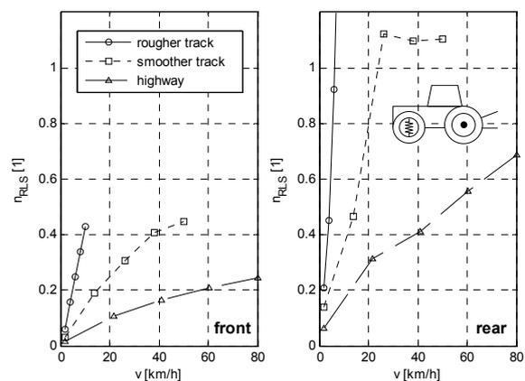
Figure 14: Calculated dynamic wheel load factor of the tractor model with unsprung rear axle, without rear-mounted mass.
