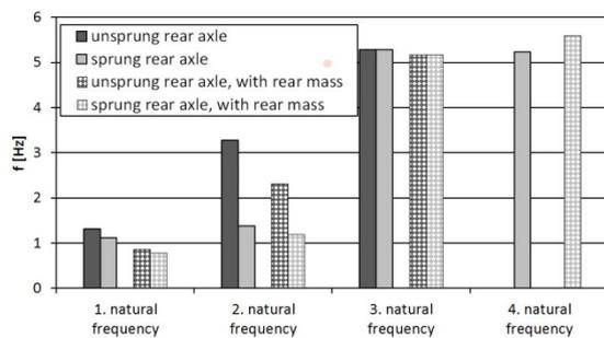
Figure 12: Overview of the first three (four) calculated natural frequencies of the tractor model showing the influence of the rear axle suspension and a rear-mounted mass.
