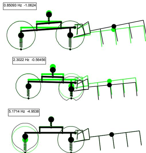
Figure 11: First three calculated eigenmodes of the tractor model with an unsprung rear axle and rear mounted mass.
