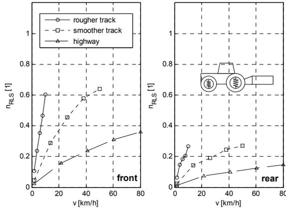
Figure 15: Calculated dynamic wheel load factor of the tractor model with sprung rear axle and rear-mounted mass.
