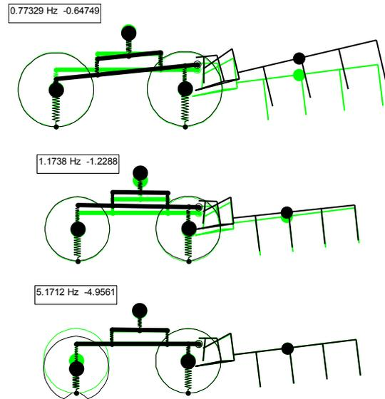
Figure 10: First three calculated eigenmodes of the tractor model with a sprung rear axle and rear mounted mass.
