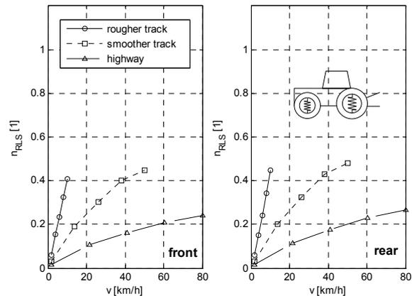
Figure 13: Calculated dynamic wheel load factor of the tractor model with sprung rear axle, without rear-mounted mass.
