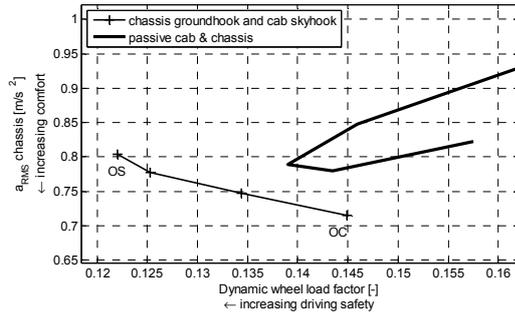
Figure 4: Comparison of passive cabin and axle suspension and skyhook-controlled cabin suspension with groundhook-controlled axle suspension on the ISO 5008 smoother track.
