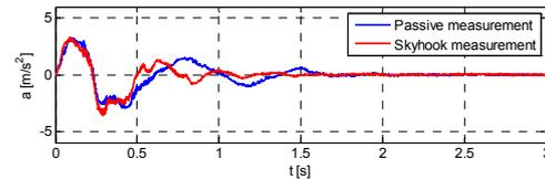
Figure 5: Step response for passive and skyhook-controlled chassis suspension.
