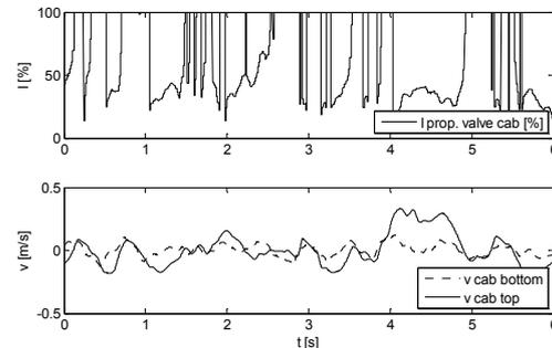
Figure 6: Actuator current and cabin suspension velocities
