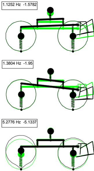
Figure 8: First three calculated eigenmodes of the tractor model with a sprung rear axle.
