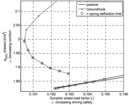
Figure 3: Comparison of passive and groundhook-controlled suspension on the ISO 5008 rougher track.
