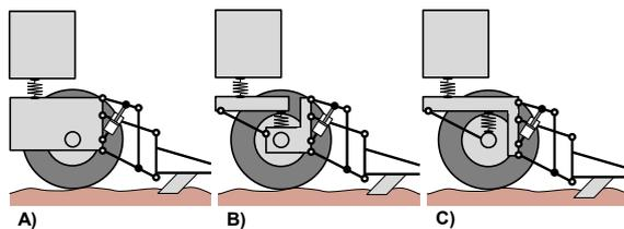
Figure 7 : Three different options to connect the rear-mounted three-point linkage to the tractor. A: directly to the unsprung chassis, B: to the sprung rear axle, C: to the suspended chassis (TUB-Trac).
