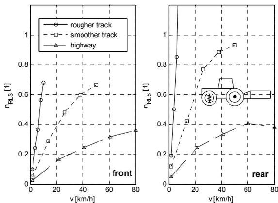
Figure 16: Calculated dynamic wheel load factor of the tractor model with an unsprung rear axle and rear-mounted mass.
