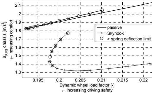
Figure 2: Comparison of passive and skyhook-controlled suspension on the ISO 5008 rougher track.
