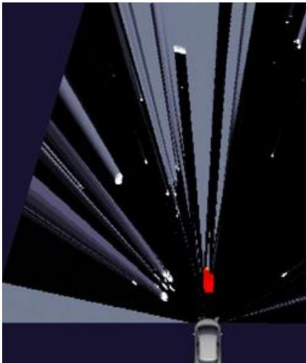
Figure 18: Filtered occupancy grid constructed from lidar data.
