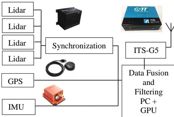
Figure 6: System architecture of our intelligent vehicle.
