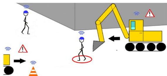
Figure 13: Example of a construction site equipped with connected devices in worker hats, vehicles and traffic cones. The digger on the right is warned by the presence of
